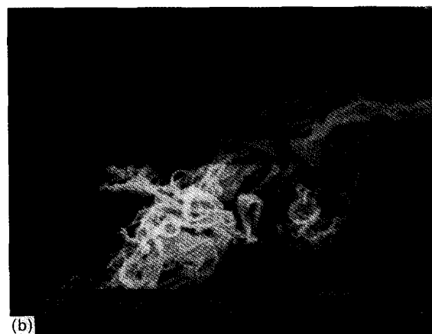
Figure 8 SEM micrographs of PAN fibrils formed by spraying a 1.8% PAN in DMF solution through a 50 \mu\text{m} i.d., 2.5 cm long nozzle into CO 2 at 40°C, 0.66 g ml -1 : (a) 0.2 ml min -1 ; (b) 2.0 ml min -1
